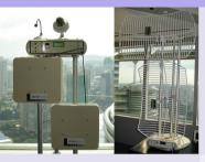
TRIATA provides a "triple play" communications system where video, voice and data can be transmitted over the same wireless link connection. The wireless link connection is deployed by using a novel technique called Pseudo-random Polarization Hopping (PPH) to provide an extremely secure anti jamming broadband wireless to overcome the threats of eavesdropping and jamming.
